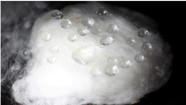
Fig 2: This picture shows the interaction between natural hydrophobic fibres and water.
