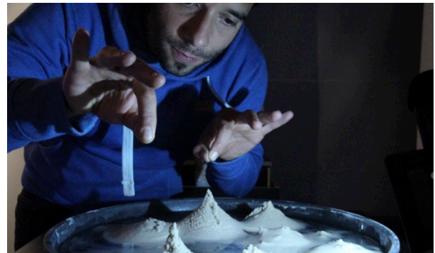
Fig 4: In this experiment, the student discovers how water can act as glue between the grains of a pile of sand, thought the capillary action of hydric forces.
